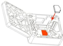
1. Remove the double-side-glued pad from the gimbal box and paste the pad into the drone's case as showing to the left.
