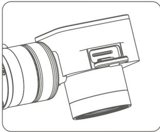
1. Open the soft rubber seal on the top of the camera, insert the Micro SD card in the correct direction, press the Micro SD card, the "click" sound indicates that the installation is in place.
